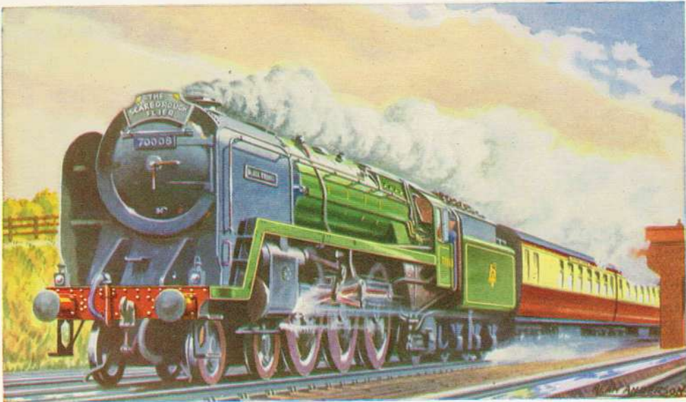
4-6-2 No. 70008 'Black Prince' Class 7-MT 'Britannia' Class. British Railways. Driving wheels 6' 2". Two cylinders 20" diam. x 28" stroke. Boiler pressure 250 lb/in 2 . Tractive effort 32,150 lb.
